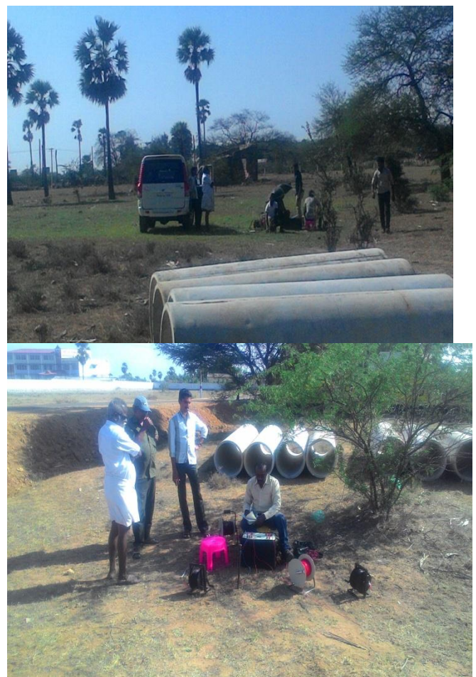
Figure.3. Show the Electrical Resistivity data collection for groundwater.
