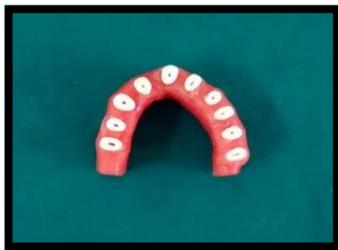
**Fig. 2)** Teeth mounted in modelling wax to simulate jaw
