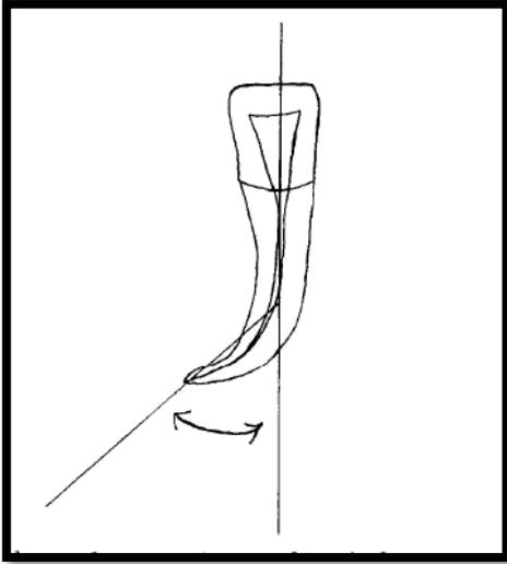
**Fig. 1)** Schneider's method for measurement of root curv
